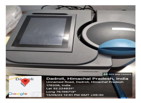
**Principle-** The principle of uv-visible spectroscopy is based on the absorption of ultraviolet light or visible light by chemical compounds, which results in the production of distinct spectra. <u>Spectroscopy</u> is based on the interaction between light and matter.
