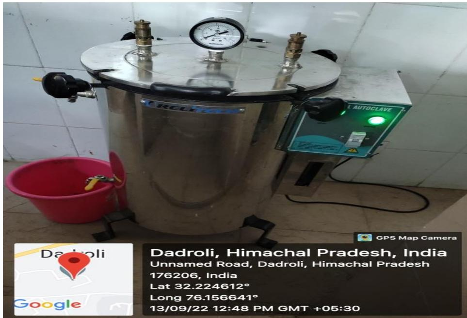
**Principle**-the autoclave works on the **principle** of moist heat sterilization. The high pressure inside the chamber increases the boiling point of water for the sterilization of equipment. The higher pressure also ensures the rapid penetration of heat into the deeper parts of equipment. The moisture present in the steam causes coagulation of proteins of microbes causing irreversible loss of their activity and functions.
