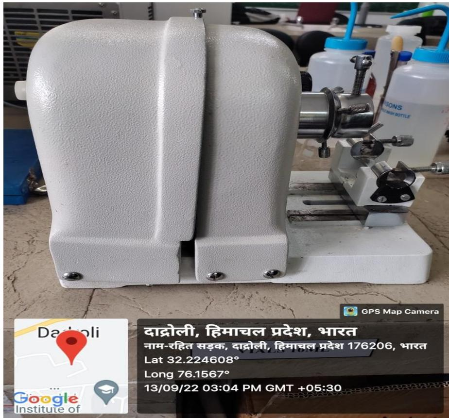
**Principle and application:** Microtome is an instrument with the help of which sections of tissues are cut and the process of cutting thin sections is known as [microtomy](#). The thickness of sections produced during microtomy may be between fractions of 50-100 nm, in ultramicrotomy, to several 100 microns.
