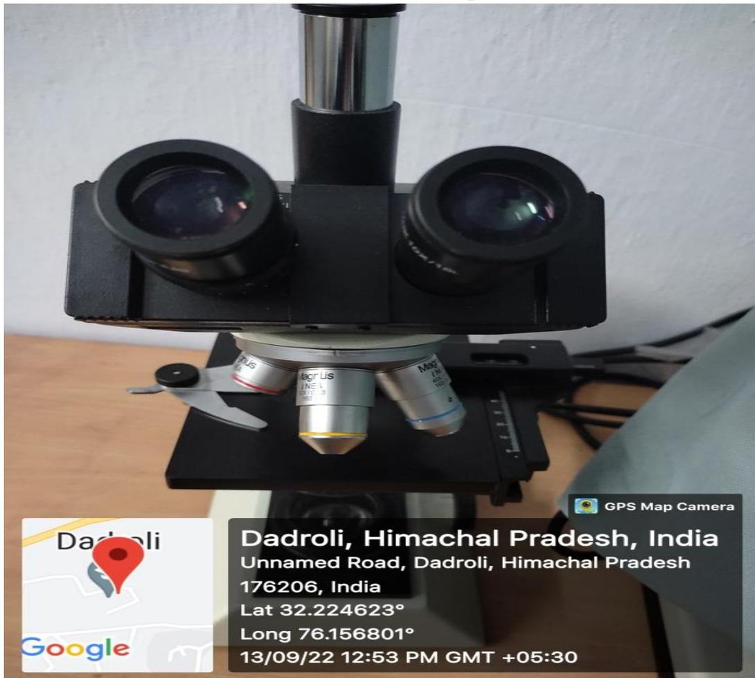
**Principle** a stereo or a dissecting microscope uses reflected light from the object. It magnifies at a low power hence ideal for amplifying opaque objects.
