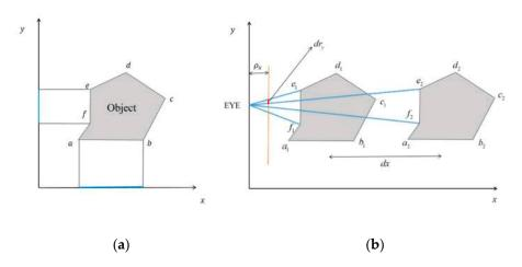
**Figure 2.** (a) A 2-D object (polygon) in the x - y coordinate system; (b) change in apparent size of the edge *ef* for a dx movement along the x axis.
